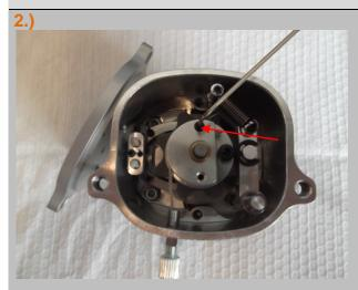
Loosen the cable retaining screw and remove the defective cable.
