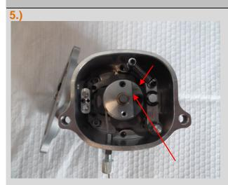
The end of the cable must protrude around 2-4 mm beyond the marked edge.
