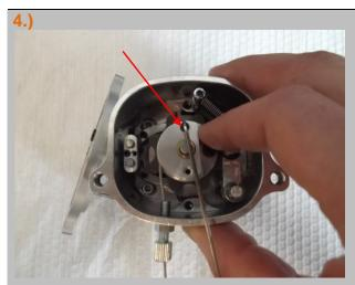
Use a finger to insert the cable along contour and tighten clamp screw.
